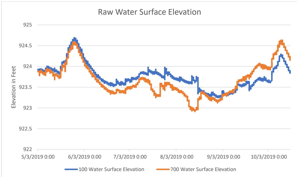
**Figure 30. Surface Water Elevations at Station 100 and 700**
