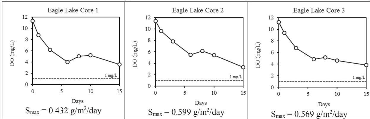
**Figure 4. Dissolved oxygen (DO) concentrations in the unmixed water columns of the Eagle Lake sediment cores during the second phase (no aeration) of the phosphorus release study. The 1 mg/L reference line for anoxia is shown as dashed line in the plots.  $S_{max}$  is the calculated sediment oxygen demand.**
