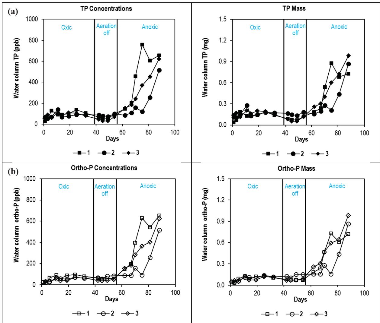
**Figure 3.** Water column concentrations and mass of (a) total phosphorus (TP), and (b) ortho-phosphate (ortho-P) in the Eagle Lake sediment cores during the phosphorus release study. The three phases of the study are separated by solid vertical lines (oxic = aeration on; anoxic = N<sub>2</sub> bubbling on).
